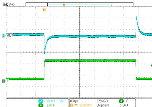
Figure 12. Load Transient
