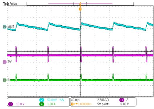
Figure 11. SW node Waveform and Output Ripple, IOUT=10mA
