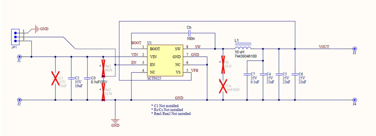
Figure 3. SCT9325 Evaluation Board Schematic
