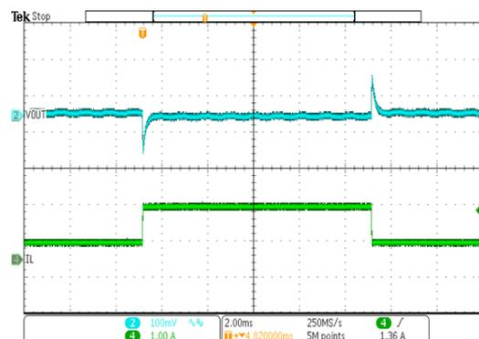
Figure 13. Load Transient
