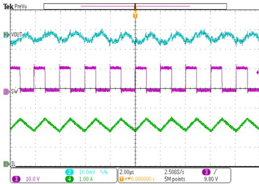
Figure 10. SW node waveform and Output Ripple, IOUT=2A
