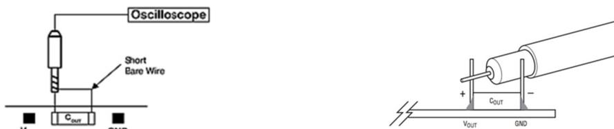
Figure 2. Measuring Voltage Ripple Across Terminals or Directly Across Ceramic Capacitor
