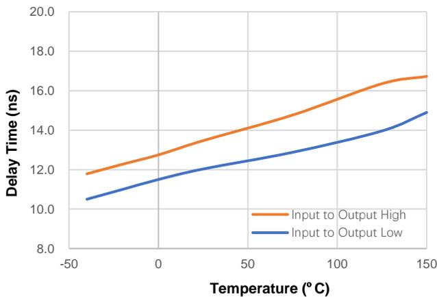
Figure 5. Input to Output Propagation Delay vs Temperature
