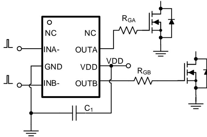
Figure 16. Dual Channel Driver Typical Application
