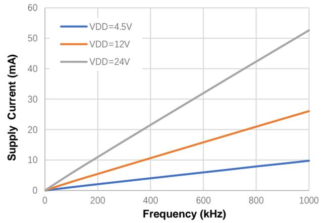
Figure 8. Operation Supply Current vs Frequency,  $C_{OUT}=1nF$
