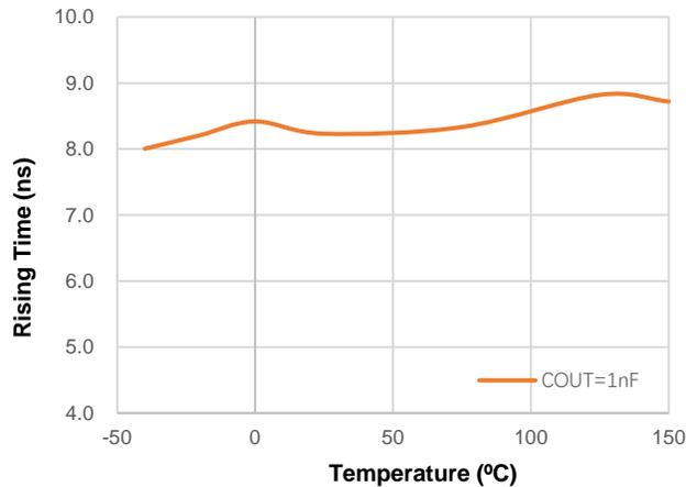
Figure 3. Output Rising Time vs Temperature
