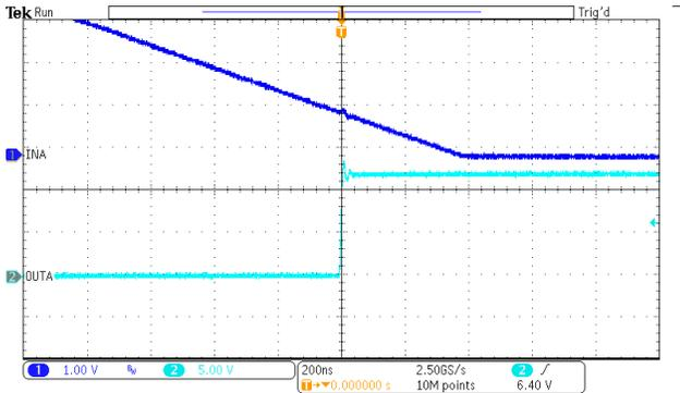
Figure 14. Driver Switching ON
